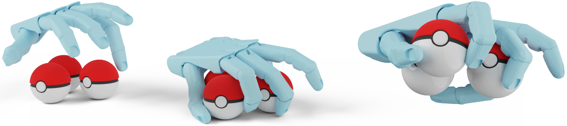
Fig. 1: The proposed multi-object grasping method, MultiGrasp , drives the Shadow Hand to simultaneously grasp multiple Pokémons.
